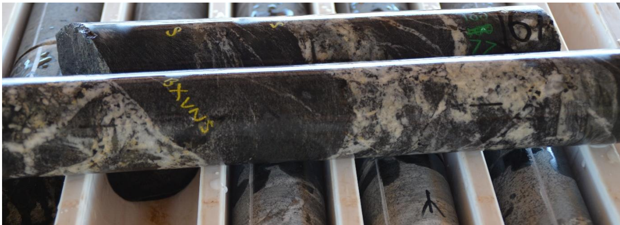
DKRC0007 67m – Quartz-carbonate-sulphide-tourmaline brecciated veins in strongly foliated gabbro
