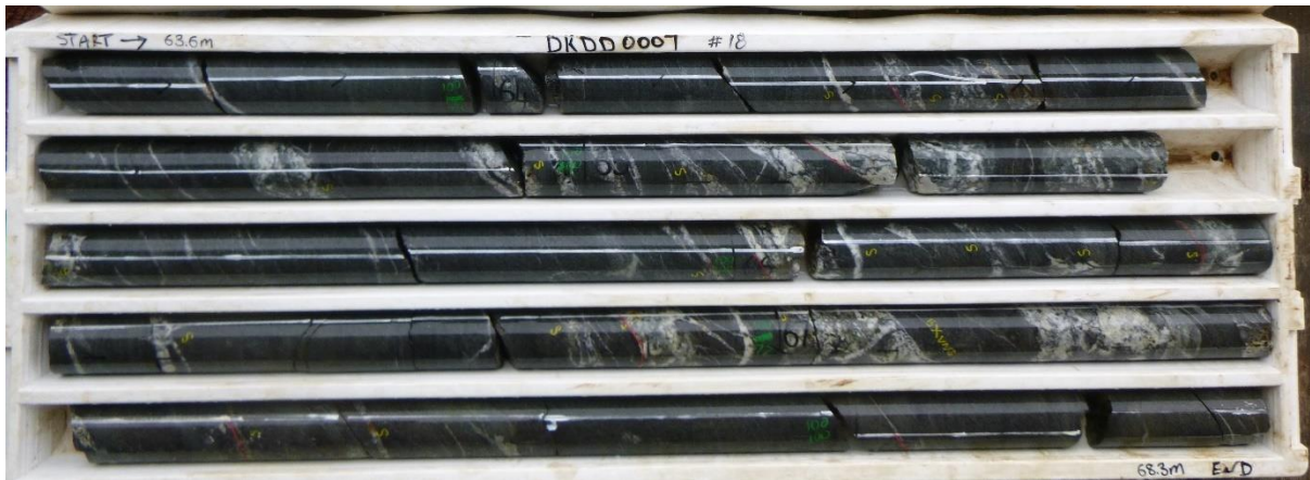
DKDD0007 63.6-68.3m – multiple quartz-sulphide-carbonate vein sets within a strongly foliated gabbro.
